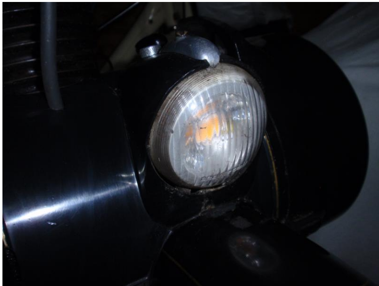
The yellow LED circuit almost looks like the original yellow tinted globe.
